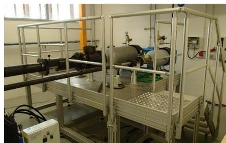
*High velocity impact test platform shared with the Institut Clément Ader.*
