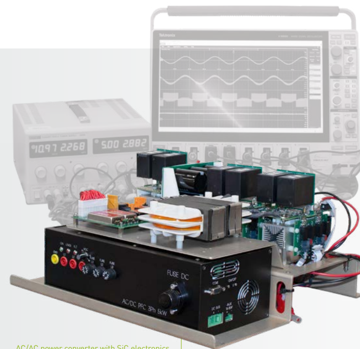
AC/AC power converter with SiC electronics © IRT Saint Exupéry
