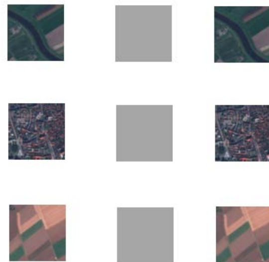
Left Column - An image well classified by the neural network Center Column - A tiny perturbation created specifically using the image on the left Right Column - The resulting perturbed image wrongly classified. Even imperceptible perturbation can deceive the neural network © IRT Saint Exupéry
