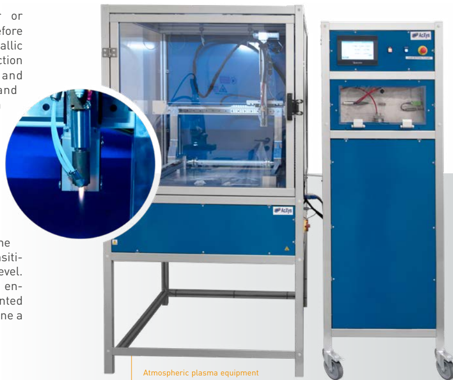
Atmospheric plasma equipment for surface preparation
