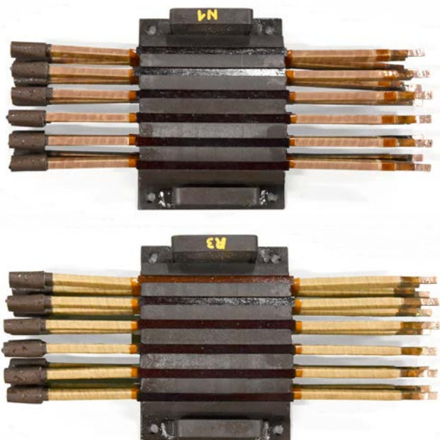
Picture of a formed wound motorette to be characterized under ageing due to partial discharge © IRT Saint Exupéry
