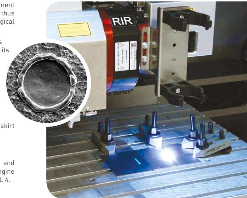
UV & IR Lasers equipment for surface preparation
