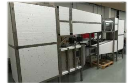
Icing Wind Tunnel (ICA)
