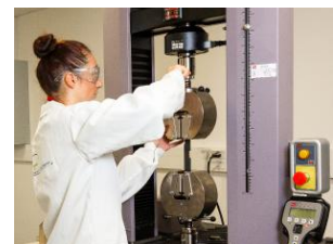
Static Mechanical test device MTS criterion C43.504 (50KN)
