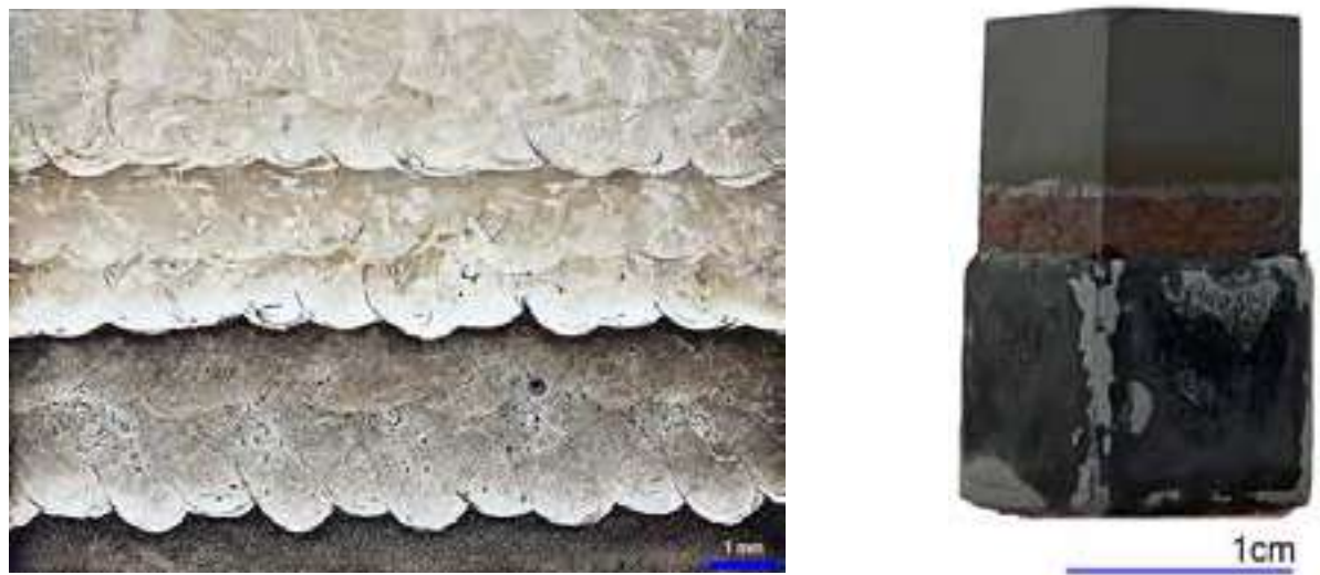
Example of gradient materials developed by LMD (Laser Metal Deposition) and characterized in the framework of Agathe Curnis' thesis (supervision Aurélien Prillieux - IRT, Ioana Popa - ICB, Sébastien Chevalier - ICB)
