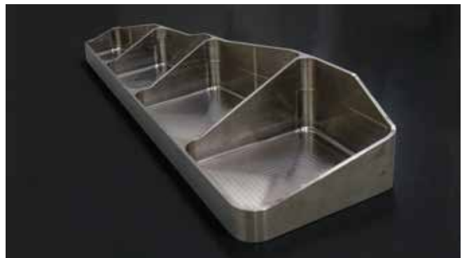
Figure 5 - Same section after finish machining
