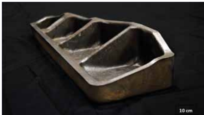
Figure 4 - representative section of an Airbus A350 fuselage frame, TRL 5 & TRL6
